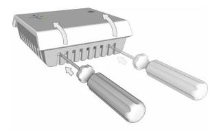
Continue to move the upper part with all the electronics until it is separated from the lower part.
