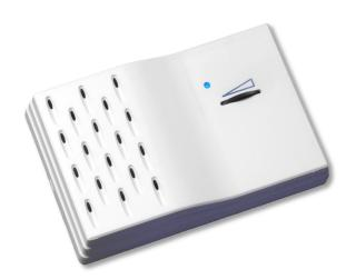
ADS-RH is a capacitive relative humidity (RH) sensor. It is equipped with an output relay with adjustable switching level and with 0 - 10 V analog output. The measurement is performed periodically after about 7s. Based on these measurements it is possible to directly control the ventilation, air conditioning and heat recovery units.
