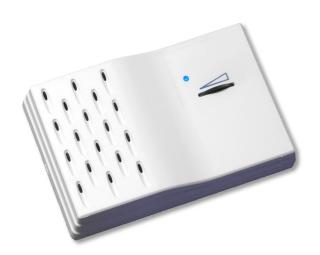
ADS-RH is a capacitive relative humidity (RH) sensor. It is equipped with a 0-10V analog output and with an output relay with adjustable switching level. The measurement is performed periodically after about 7s. Based on these measurements it is possible to directly control the ventilation, air conditioning and heat recovery units.
