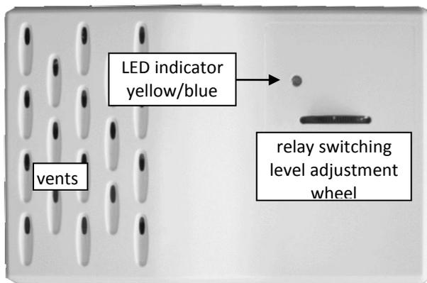
**Relay switching level adjustment wheel:**
