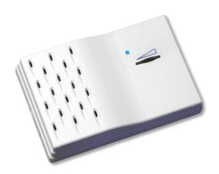
ADS-SMOKE is an indoor air quality sensor with analog voltage output 0 - 10 V and an output relay with adjustable switching level. The sensor has a high sensitivity to low concentrations of pollutant gasses in the air. For example carbon monoxide and hydrogen, those are contained in the cigarette smoke. Therefore is the ADS-SMOKE appropriate for use in areas polluted by cigarette smoke. Monitoring of the air pollution allows very economical controlling of ventilation systems.
